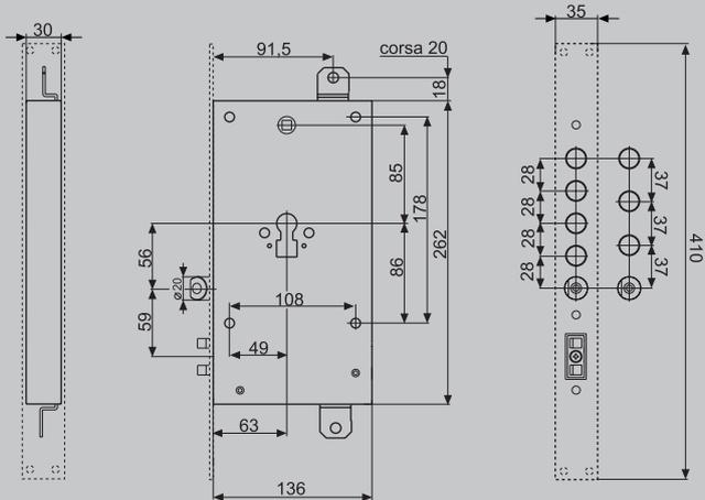
The new FIAM x1R electronic locks are interchangeable with dimensional standards adopted for most common mechanical locks, have the same range of accessories and the electrical connections required, both during construction of the door and during installation, are much simpler than you would think at this moment in time...
